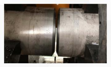
Cut off + beveling synchronous processing
